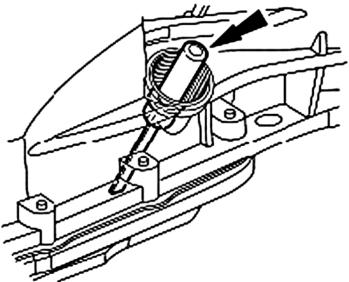
• Remove the dipstick and read the level.
