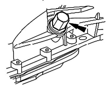
• Remove the dipstick from the fill cap.
