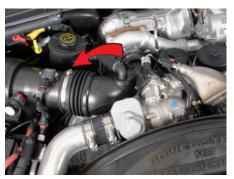
6. Loosen the clamp on the intake hose and carefully disconnect the hose from the throttle body.
