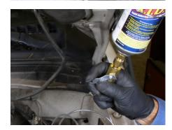
9. Open the valve slowly to release the cleaner a little at a time. If the engine begins to race or run rough, close the valve a little.
