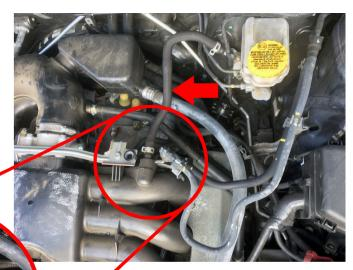
This brake booster vacuum hose connects to a single rail on the intake manifold, so the cleaning detergent won't reach the rest of the cylinders. The result is improper cleaning, and possible engine damage.
