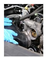
1. Disconnect the air inlet boot past the mass airflow sensor, as close to the throttle body as possible.
