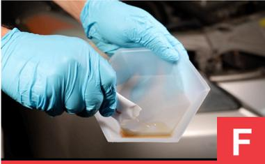
F. Open package of Step 2 Lens Refinisher. Pour it into clean tray.
