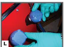
11. When the differential is full, close the ball valve. Remove wand Replace and tighten differential drain plug.
