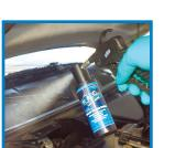
STEP 2: Close all windows; remove pets and people from the vehicle and start engine. Set A/C controls to normal on position, fan on high. Set selector to Outside or Fresh Air, close doors.
