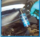
**STEP 3: Under the Hood, locate exterior air intake** (usually at base of windshield), aim F.A.Q. Spray Gun at air intake and spray liberally into air intake for 50-60 seconds.
