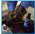
Replacing the Cabin Air Filter: **Follow** manufacturer's instructions for removing cabin air filter but DO NOT install new filter until the F.A.Q. service is completed! After removing the filter, proceed to Step 1.
