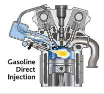
In G.D.I. engines the injector position does not allow gasoline or fuel additives the ability to wash dirt & deposits away during engine operation. Without a professional cleaning, there is no way to deliver detergent to clean the dry induction system. This results in poor engine performance.
