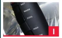
I. The coating will dry in 30 – 40 minutes, yet the vehicle can be driven right away. To speed the drying process, use a COOL air hair dryer only! DO NOT USE A HEAT GUN. Avoid touching the lens or using a car wash for 24 hours.
