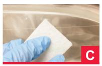
C. Next, spray the pad once or twice and scrub the lens surface with the cleaner/prep pad vigorously. This will remove the damaged coating.
