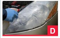
D. Now, completely clean the lens by wiping with a clean paper towel, then spray the lens with water and wipe it completely clean. Use another towel to dry the lens.
