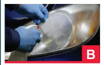
B. Prep both headlights by applying the Lens Cleaner to the surface of the lens. Apply a coating of the prep to each lens. Allow the Prep to stay on the lens for at least 30 seconds. It will start to soften and remove discoloration.
